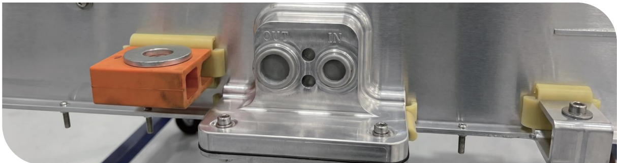
Battery Pack Refrigerant Port
